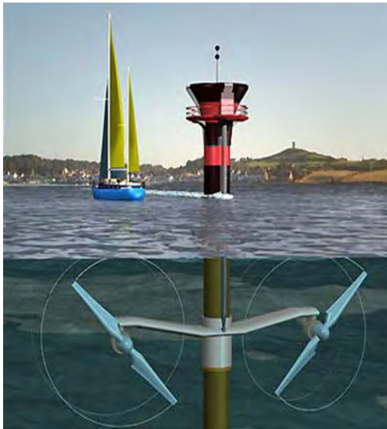
This image shows water turbines installed inside the barrage, and wings rotating with the flow of water to produce electricity
